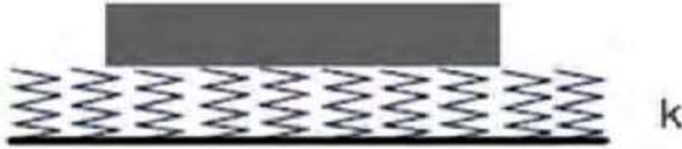
Fig. 1: Slab on Winkler (DL) Foundation Type Area
