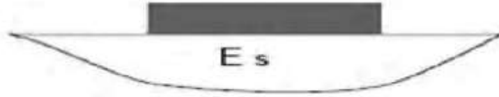
Fig. 2: Slab on Elastic Solid (ES) Foundation
