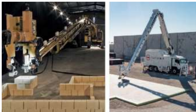
Fig. 1.5: Hadrian 105 prototype (left) and successor version - Hadrian X (right) by Fastbrick Robotics: a one-armed robot for the construction of structurally sound brick walls on site. (Dörfler, 2018)
