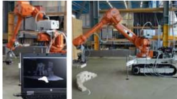
Fig. 1.6: DimRob, the first mobile construction robot prototype of Gramazio Kohler Research presented in 2012. (Dörfler, 2018)
