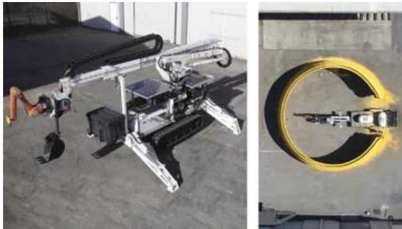
Fig. 1.4: The DCP (Digital Construction Platform) (left). In 2017, the system fabricated a stay-in-place formwork for an open dome-like structure. (Dörfler, 2018)
