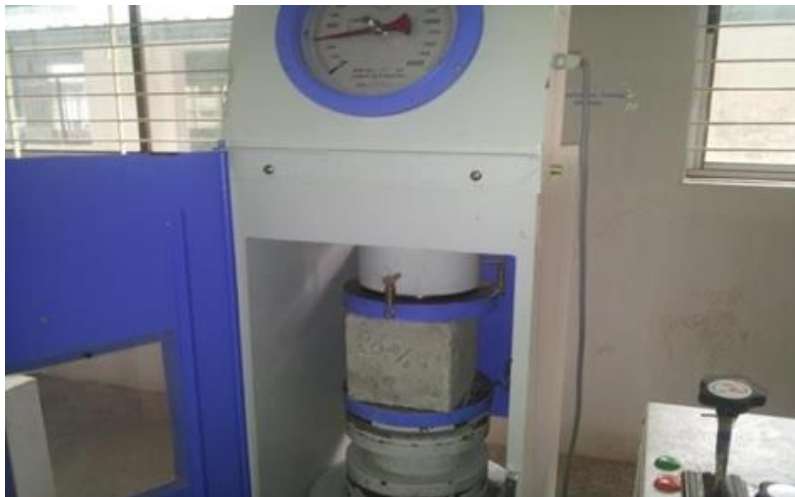
FIG II. COMPRESSIVE STRENGTH TEST
