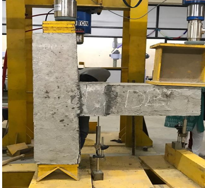
Figure 7: Precast Connection using Couplers test set up
