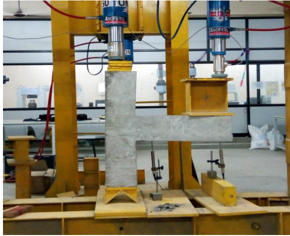
Figure 4: Monolithic Connection Testing set up
