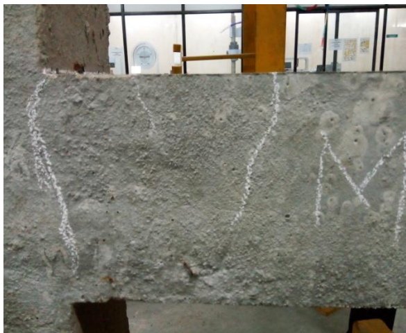
Figure 5: Crack formation in Monolithic Connection
