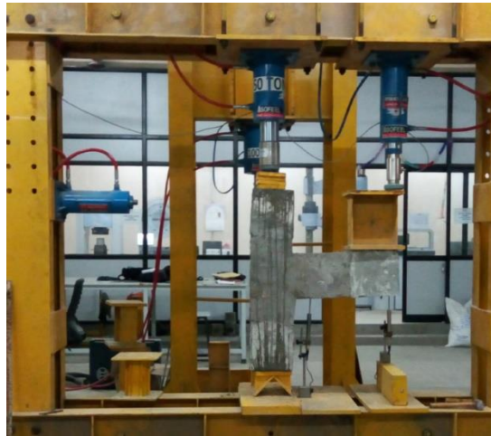
Figure 10: Precast connection using MS Pipes testing set up
