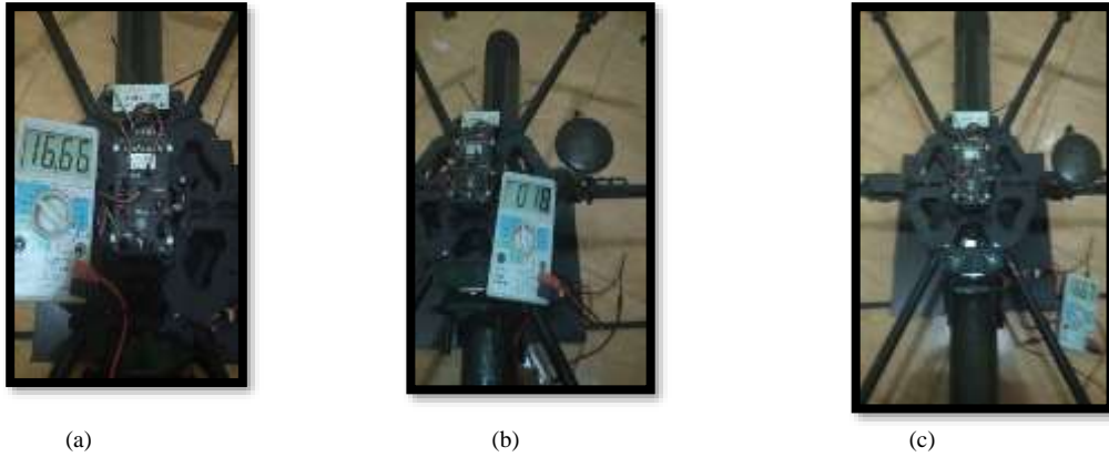
Figure 17. Voltage Measurement (a) FCS (b) ESC (c) Trigger Circuit
