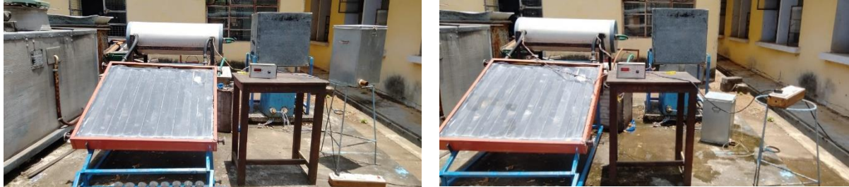
Figure. 7.1: Temperature difference of solar water heater with and without PCM in solar collector
