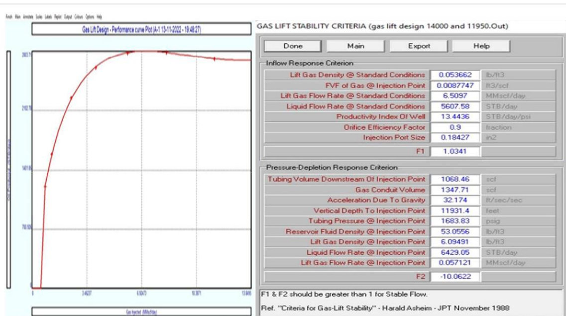
Figure 9 (a) Gas lift: Performance Curve (b) Gas Lift: To check Stability Criteria
