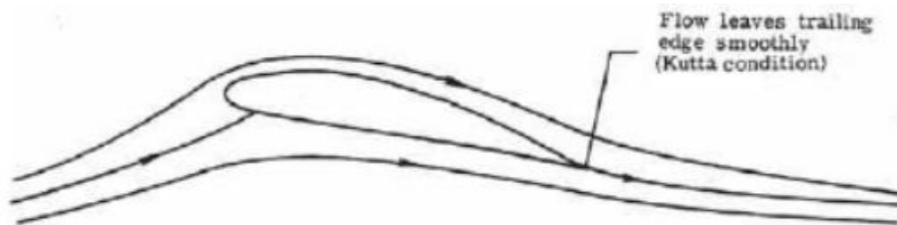
Figure 2: Inviscid flow over an airfoil with the Kutta condition satisfied. The flow meets smoothly at the trailing edge. (Milne-Thomson, 1958).
