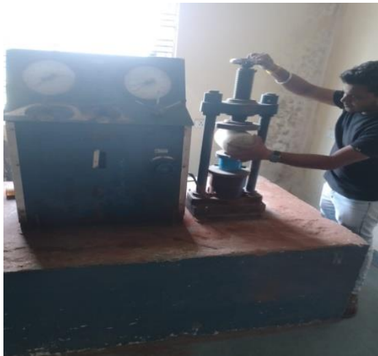
Figure:3 Split Tensile Strength Test during lab days and 28 days
