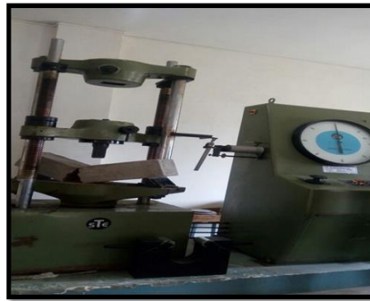
Figure 2 Flexural Strength Testing on Specimen Using UTM
