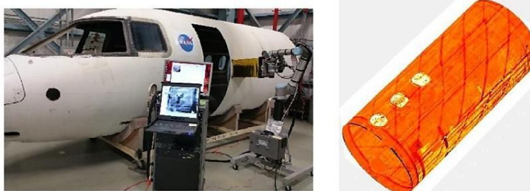
Fig. 22- IRT of aircraft fuselage and its 3D view of thermal data [80]
