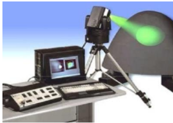
Fig. 26- Shearography (LTI) Image in aviation [104]
