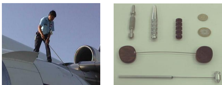
Fig. 6–Aviation Tap Testing at Maintenance Depot [36]
