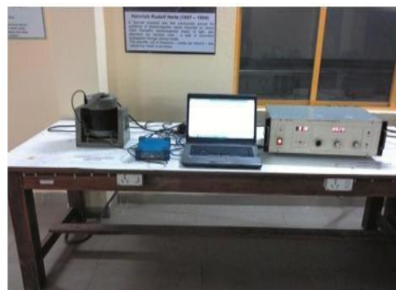
Fig. 16 – Researchers' setup for vibration test of carbon fiber beam [59]
