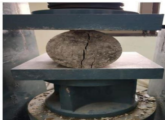
Figure 2 Split tensile strength test under CTM
