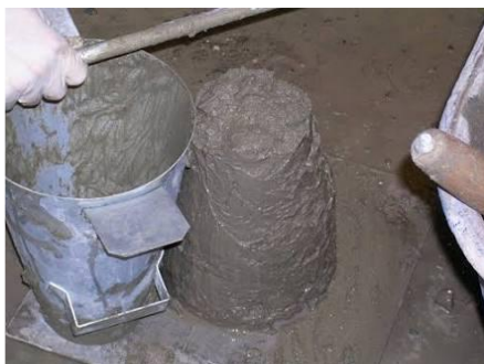
Figure Slump Test of Concrete
