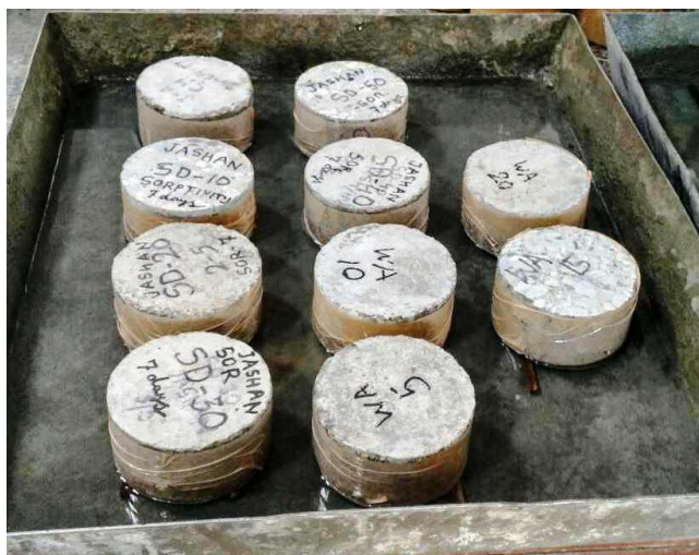
Figure : Sorptivity Test of Concrete Samples
