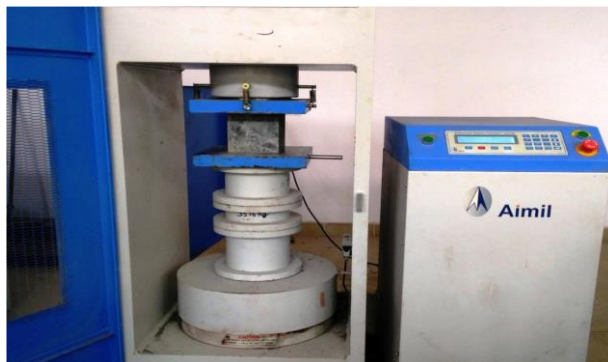
Figure : Compressive Strength Test on Compression Testing Machine
