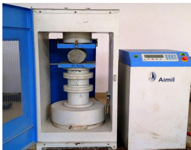
Fig. Splitting Tensile Strength Test of Concrete
