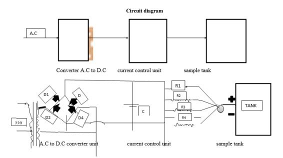
Figure 1 Circuit diagram of electrophoresis machine
