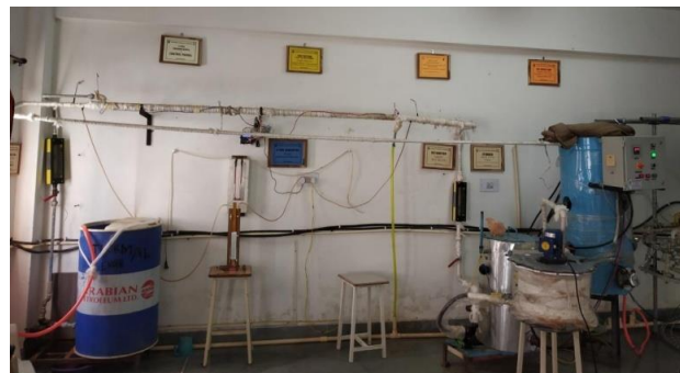
Figure 6 : Experimental setup for DPHE in Heat Transfer Research Lab
