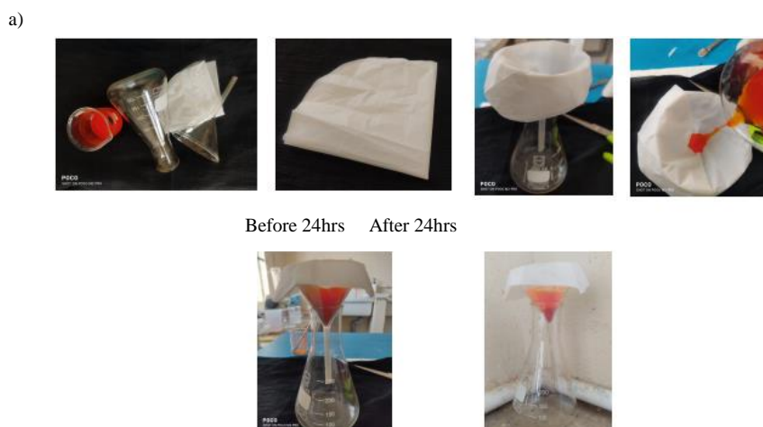
Figure 4 - (a) Leakage proof test.
