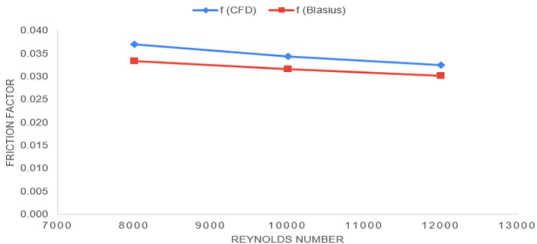
Figure 4.2.2 f calculated with CFD vs f calculated with Blasius equation
