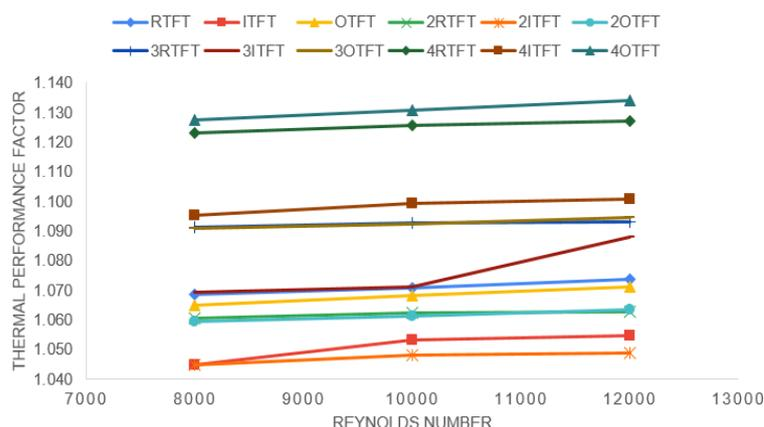
Figure 4.3.3 Thermal performance factor ( $\eta$ ) vs  $Re$  for the finned tubes
