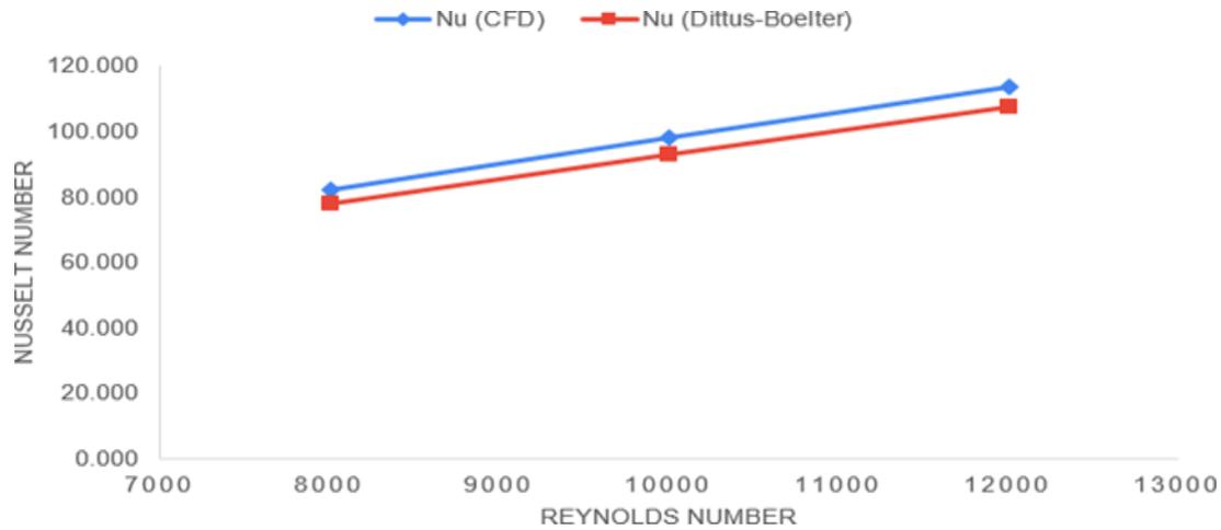
Figure 4.2.1 Nu calculated with CFD vs Nu calculated with Dittus-Boelter equation
