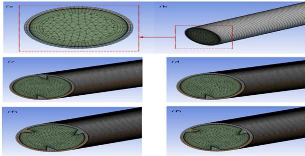
Figure 3.4.1 represents a sample of meshes that were generated for the plain tube (PT) and the tubes equipped with one, two, three and four right-angle triangular fins
