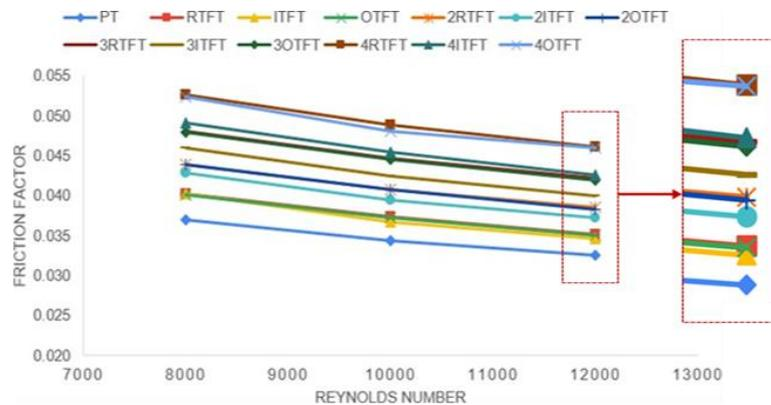
Figure 4.3.2 f vs Re for plain tube and finned tubes
