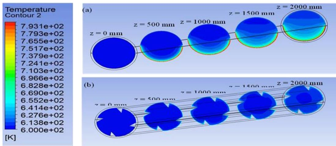
Figure 4.4.1 Temperature contour at  $Re = 12000$  for: (a) PT (b) 4RTFT
