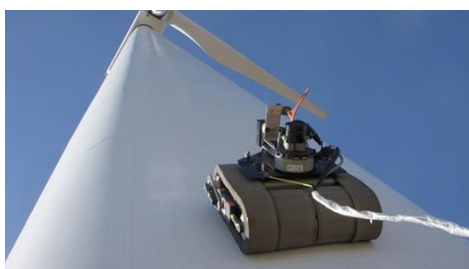
Fig. 8 Robotic crawler climbs wind turbines to inspect blades.
