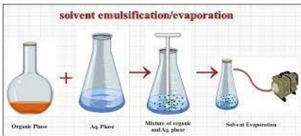
Figure-5 solvent emulsification/evaporation technique
