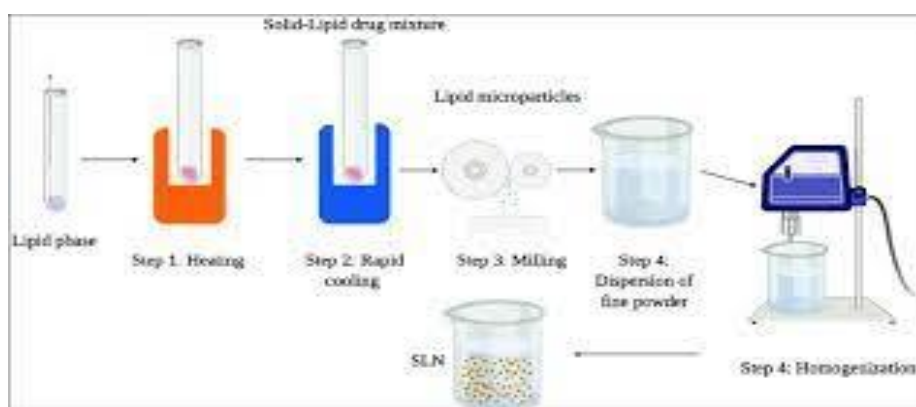
Figure-4 Cold homogenization technique
