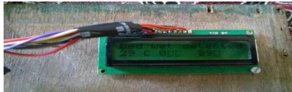
Fig.2: Bed Wet detected.
