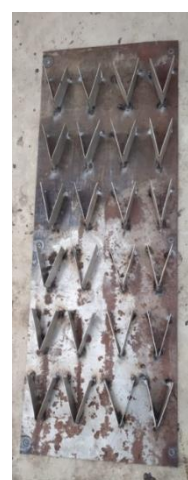
Plate 2 V Rib on Absorber Plate
