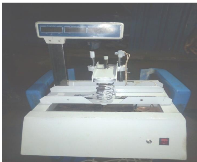
Fig. 4 – Designed and fabricated spring test apparatus
