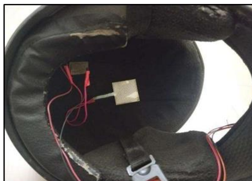
Figure 4: Positioning of FSR in the helmet
