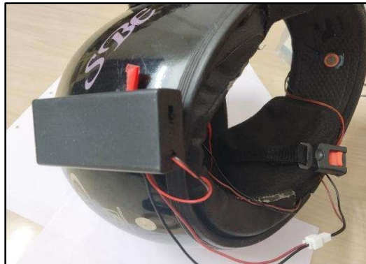
Figure 7: Mounting of battery on the helmet
