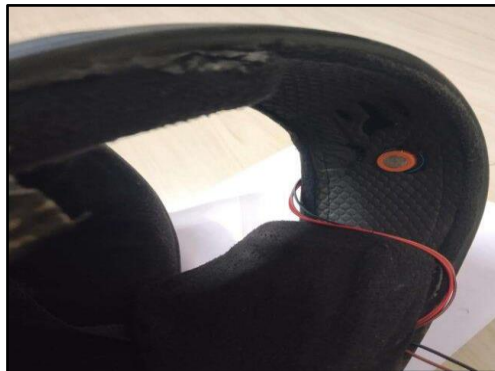
Figure 3: Positioning of alcohol sensor on helmet
