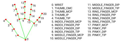
Mediapipe hands object as input and returns a dictionary containing the distance data and the original image with annotated landmarks.
