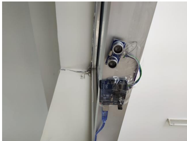
Fig. 4. Installed devices to implement security system using ultrasonic sensor and Arduino UNO.
