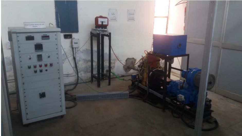
Fig 1. Test setup single cylinder VCR engine
