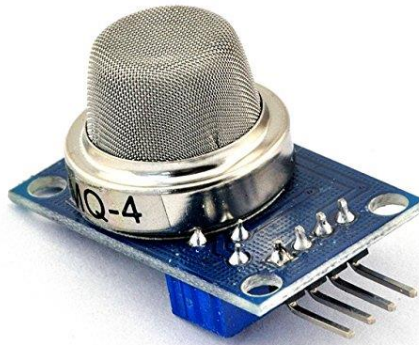
Figure 5. Spontaneous methane is detected by the detector MQ4
