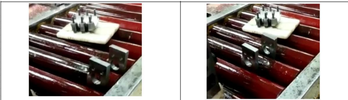
Fig:- Correct/Incorrect combination display with stopper position
