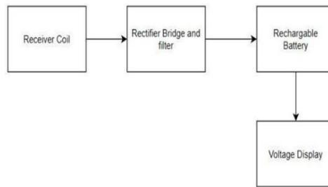
Fig 2. Receiver side block
