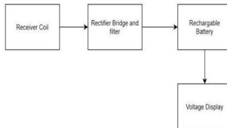
Fig 2. Receiver side block
