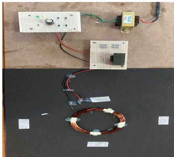
Fig.8 (b) Transmission side hardware set-up
