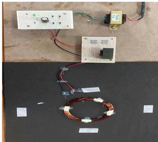
Fig.8 (b) Transmission side hardware set-up
