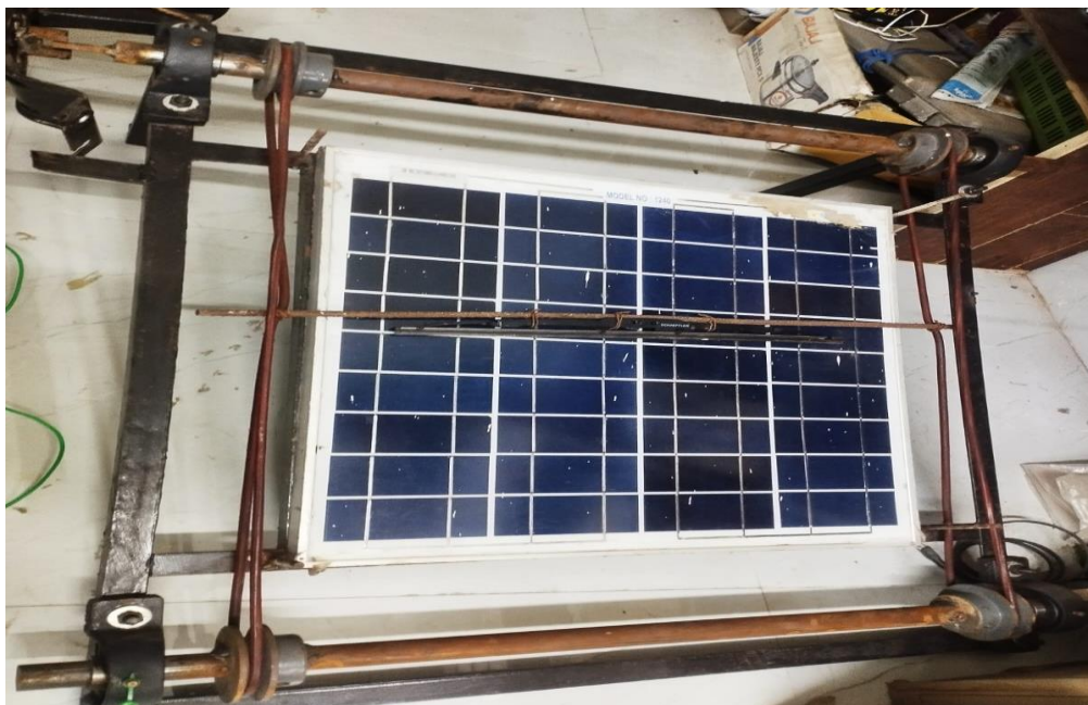
Fig:- Working model of Automatic Solar Panel Cleaning System
