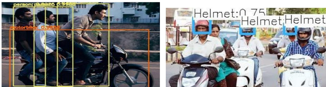
Step 2: Detection of helmet and triple riders using CNN-YoloV3
