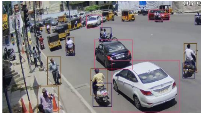
Step 1: Extraction of motorbikes from surveillance video using YoloV3 Algorithm.
