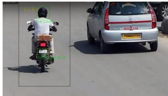
Step 2: Detection of helmet and triple riders using CNN-YoloV3
