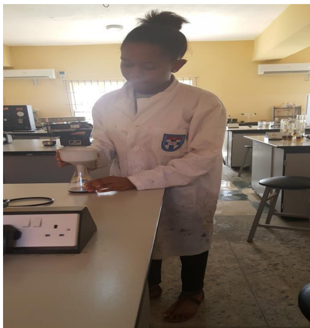
Figure 4: Separation of solid phase using a Buchner Funnel
