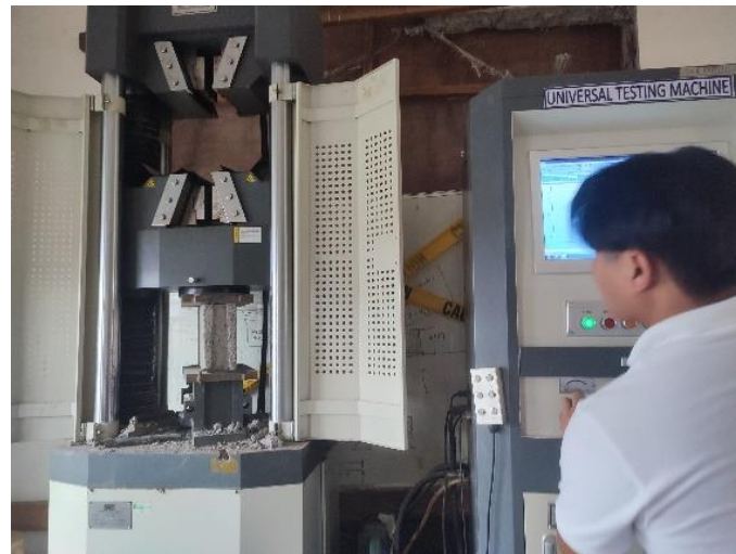
Figure 3: Compressive Strength Test Set – up
