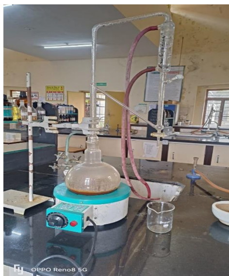
Fig.5.3: Extraction of clove oil from clove using Clevenger apparatus
