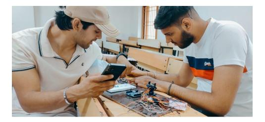
The microcontroller we used is an Arduino Uno. The Uno is a popular microcontroller board that is easy to program and has a wide range of input and output pins. We programmed the Uno using the Arduino Integrated Development Environment (IDE). The program reads the signals from the LDRs and uses a simple algorithm to determine the position of the sun. Based on this information, the program adjusts the position of the solar panel by controlling the motor through the motor driver.
