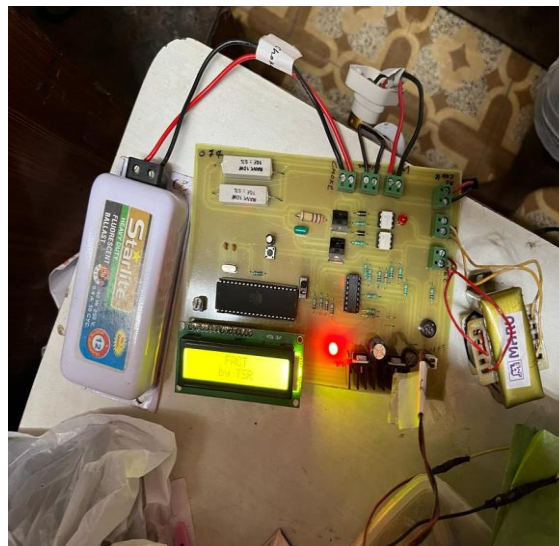
Figure 3.1: Complete Setup of Flexible AC Transmission Using TSR
