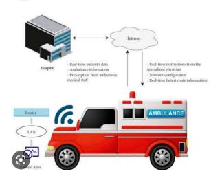
In this figure the system architecture of IOT based emergency health care monitoring system in ambulance is shown. Where in the ambulance the patient in critical situation transfer to the hospital and the doctor can get access of patient health through app in local area network which is connected through the internet. The data which is sense by the sensor is send to the nearby hospitals present in that particular area. the sender and receiver can connect and get access through the cloud.
