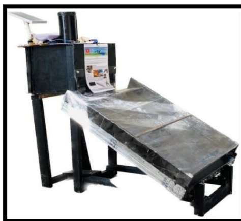
Figure 2: Actual setup of Valvular Conduits for air flow in unidirectional solar dryer.
