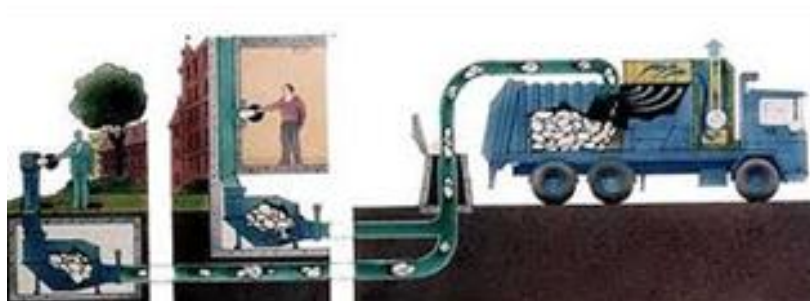
Fig. 3 - Pneumatic waste collection system.
