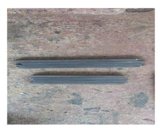
The material fits our sizing specifications. Power chop saw is the tool used for this process. A power instrument used to quickly and precisely crosscut a work item at a chosen angle is a power chop saw, sometimes referred to as a drop saw. Operations involving framing and moulding cutting are frequent uses. The majority of chop saws are compact and portable, and their typical blade diameters range from eight to twelve inches.
