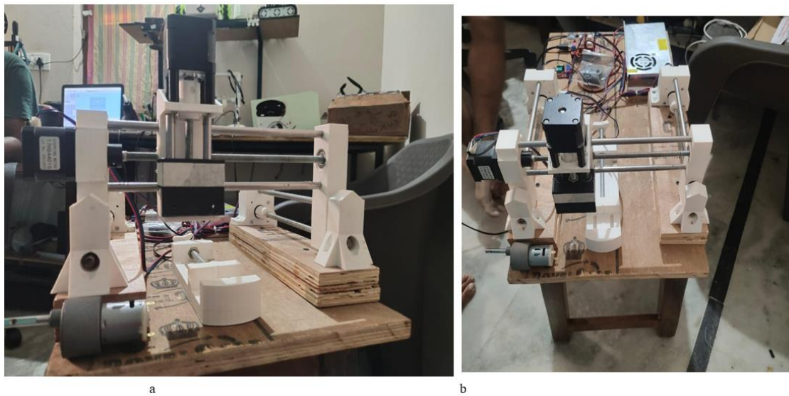
Fig 3: Four-coil configuration, (a) Coils hang under the workpiece and MAPs, (b) Coils are located above the workpiece
