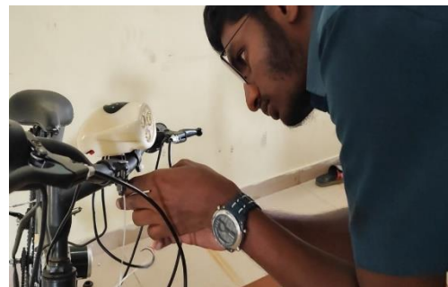
Figure 8 Installing light &amp; horn
