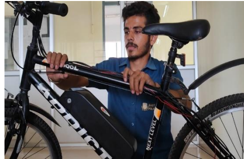
Figure 6 securing the wiring
