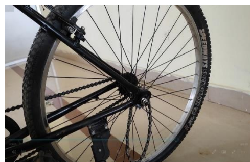
Figure 2 Installing chain to wheel sprocket
