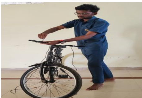
Figure 1 Installing throttle & electric brakes
