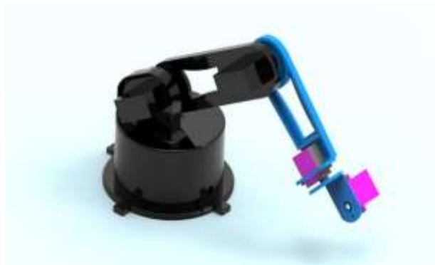
Fig.3 CAD Model of the designed robotic arm
