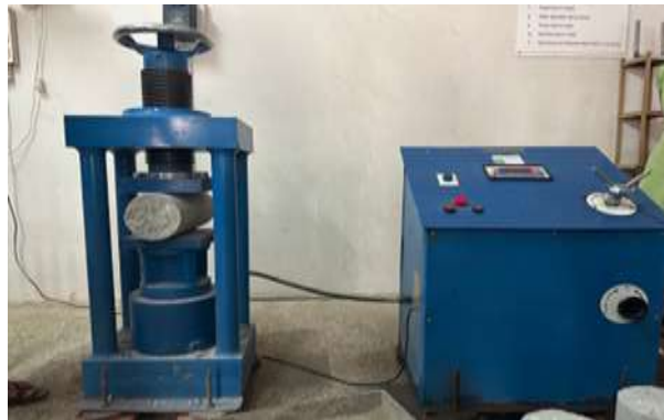
Fig. Split Tensile Strength Test on Cylinder
