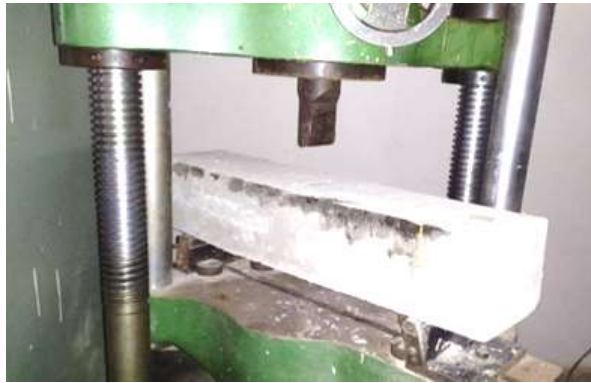
Fig. Flexural Strength Test on Beam
