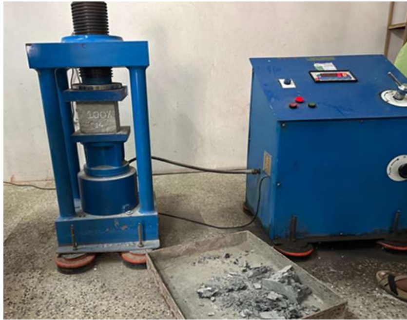
Fig. Compressive Strength Test on Concrete Cubes
