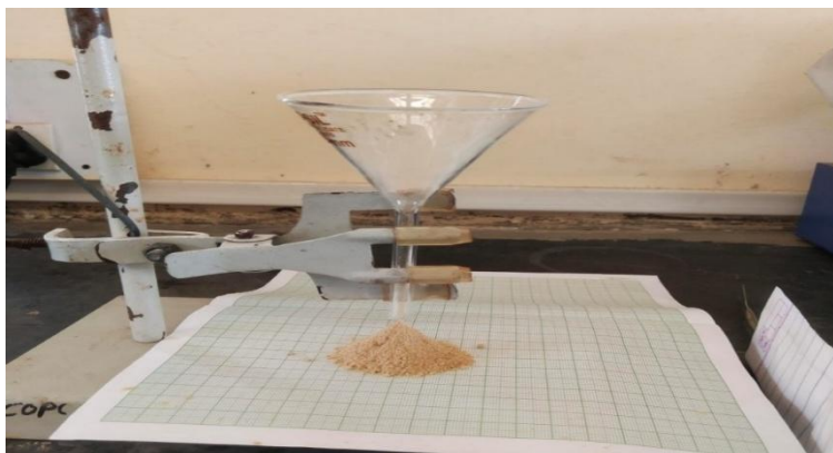
Fig No. 1. Angle of Repose
