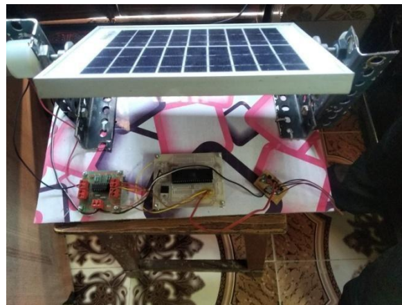
Figure 3.1: Complete Setup Of 8051 Microcontroller Based Solar Tracker System
