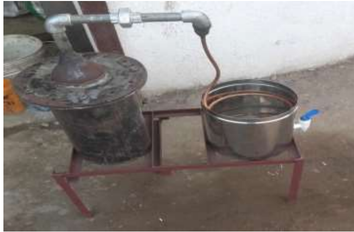
Fig.3.2. Model Of Thermofuel from Waste Plastic
