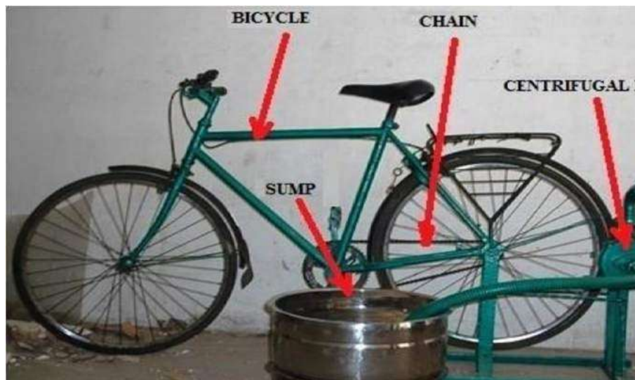
Fig- Components of pedal operated pump
