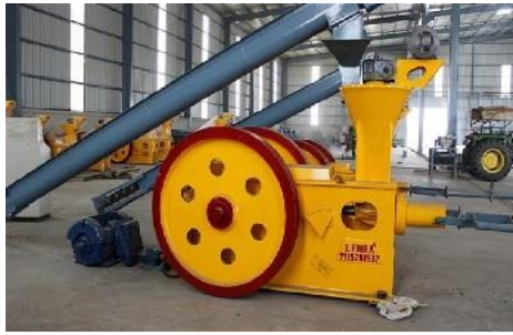
Fig. 4 Briquetting Machine at Leaf Biofuels (Source: Lehra Machinery)
