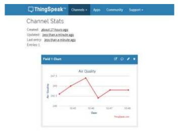
Users must log in to the ThingSpeak platform via a registered account to view and monitor sensor data. The Arduino sketch manages to read the sensor data and send AT commands to connect to the IOT platform. Learn about Arduino code from the programming guide.
